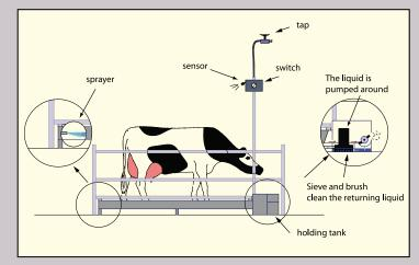
The system contains about 15 litre of liquid, which is pumped around as soon as the sensor detects the cow. Approx. 3/4 litre per cow spilled liquid will be automatically refilled.
